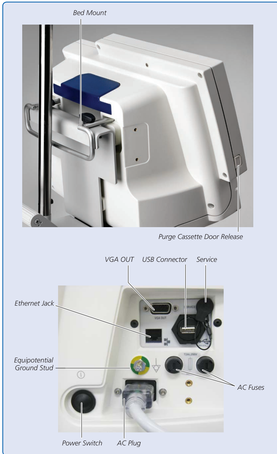
Figure 4.2 Automated Impella Controller Features – Side Views
