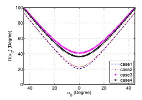
Figure 14: P&C resolution vs pointing angle. Define  $\Omega(\alpha_C)$  as  $\Omega(\alpha_C) = \max(\alpha_C) - \min(\alpha_C)$ , where  $\max(\alpha_C)$  and  $\min(\alpha_C)$  are the maximal and minimal non-distinguishable angles.
