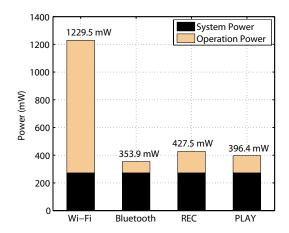
Figure 15: Power consumption of different tasks.
