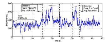
Figure 16: Power consumption of P&C procedure, excluding WiFi energy consumption.
