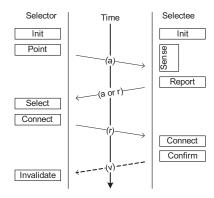
Figure 8: Block diagram of P&C, with temporal activity ordering. Characters 'a' or 'r' striking the arrows indicates the information is conveyed using acoustic or radio interface; and 'v' on dashed line implies through visual or vibration feedback.
