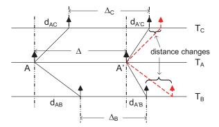
Figure 5: Illustration of the translation from maximum distance reduction to minimum interval between the two sound signals.
