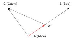
Figure 4: Principle of the P&C detection mechanism. As Alice points her phone towards Bob's, Bob sees a larger distance reduction than Cathy, as ensured by the triangular inequality:  $d_{AB} - d_{A'B} = d_{AA'} > d_{AC} - d_{A'C}$ .
