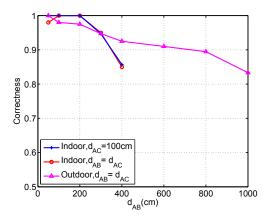
Figure 12: P&C correctness vs  $d_{AB}$ . In all cases, we fixed  $\alpha_{BC}$  to 30 degrees, and d=30cm.
