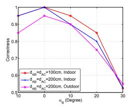
Figure 13: Resilience on pointing error. We fixed the parameters as  $d_{AB}=d_{AC}=100cm$ ,  $\alpha_{BC}=60^{\circ}$ , d=30cm.
