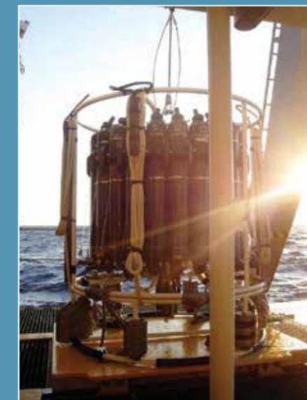
CTD rosette equipped with Niskin bottles which are used to collect seawater at various depths in the ocean.
