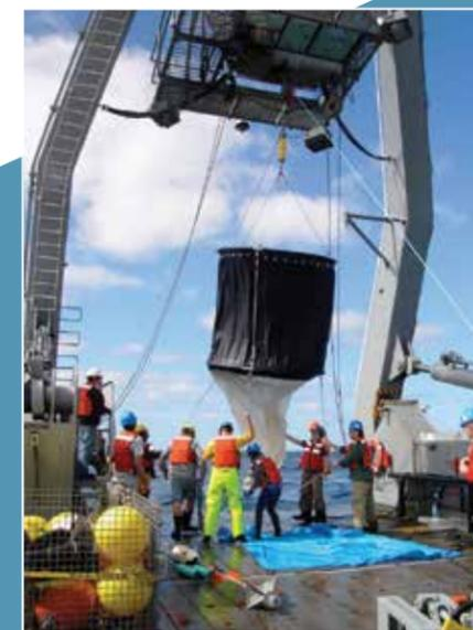
Aboard the HMS Atlantic Explorer in 2011, retrieving a surface tethered net trap that was used to collect sinking particles exported from the surface ocean to 150 m deep in the Sargasso Sea.
