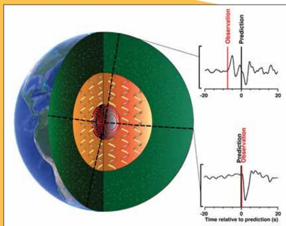
**Left:** Model of the convection in the inner and outer cores, based on seismic observations. **Right:** Seismograms demonstrating the earlier arrival of inner core waves travelling north-south relative to traveling east-west, and thus the greater wavespeed parallel to the rotation axis relative to in the equatorial plane.
