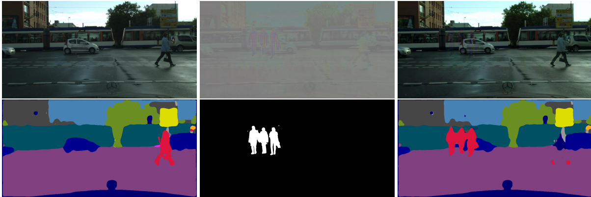
Figure 6. Type #3 attack on Cityscapes. The target ‘person’ labels disappear and the fake ‘person’ labels are embedded. Top left: The input image. Top middle: The perturbations. Top right: The input image + perturbations. Lower left: Normal predictions. Lower middle: The fake label mask. Lower right: Predictions after attacks.
