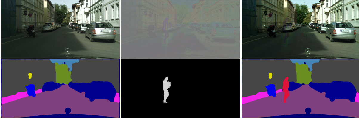
Figure 5. Type #2 attack on Cityscapes. Fake ‘person’ labels are embedded into the prediction domain. Top left: The input image. Top middle: The perturbations. Top right: The input image + perturbations. Lower left: Normal predictions. Lower middle: The fake label mask. Lower right: Predictions after attacks.
