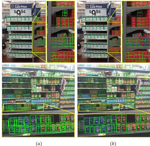
Figure 1. **Densely-packed object detection results (a) without/ (b) with the proposed HNAA attention.** Our detection method can accurately detect a large number of densely-packed small-size objects using the proposed HNAA attention.
