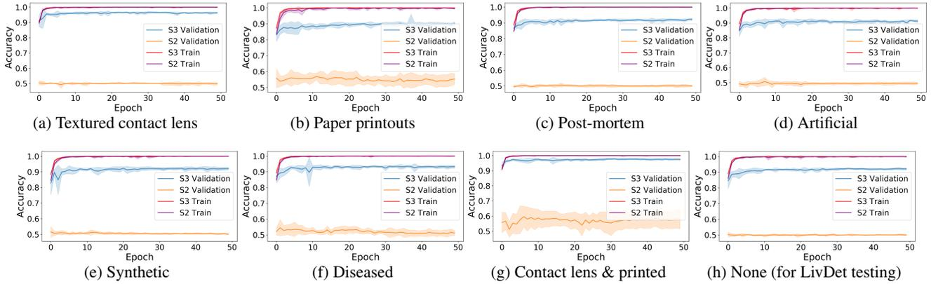
Figure 6: Accuracy on the training and validation subsets while training the models without (scenario S2) and with (S3) human saliency maps encoded into the training data. We can observe a severe overfit, and a close-to-random-chance performance of models trained without employing human intelligence (S2). In turn, human-aided saliency maps help in obtaining high validation accuracy almost instantly during training (S3).
