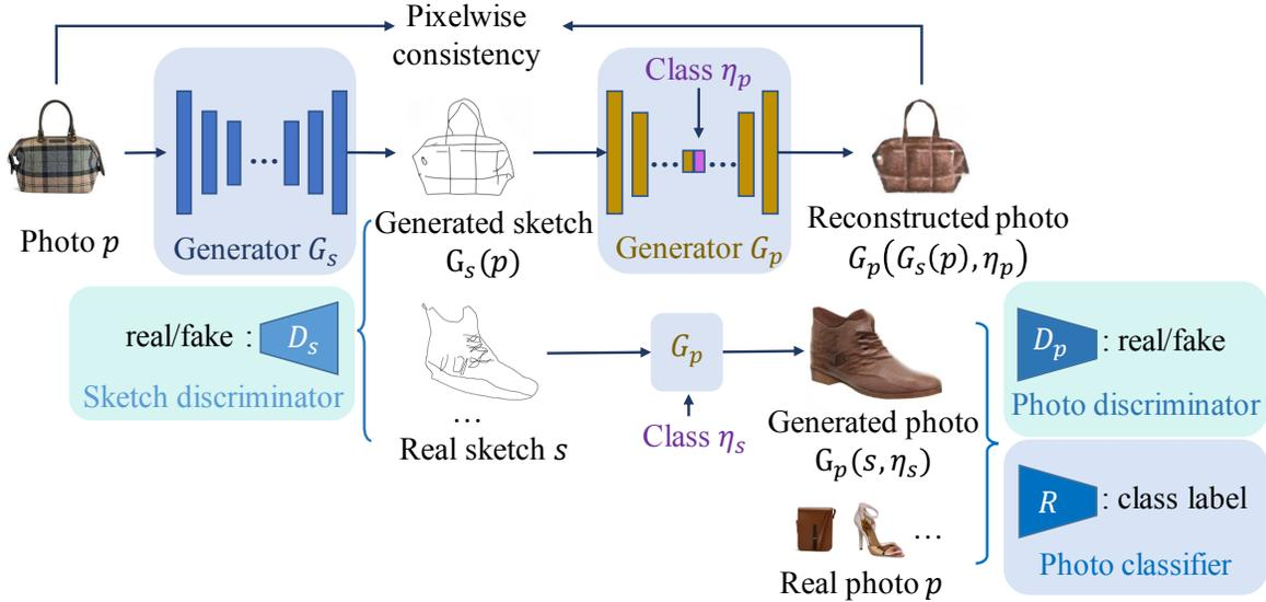
Figure 4: AODA framework overview. It has two generators  $G_s$  : photo  $\rightarrow$  sketch and  $G_p$  : sketch  $\rightarrow$  photo conditioned on the input label, and two discriminators  $D_s$  and  $D_p$  for the sketch and photo domains, respectively. In addition, we use a photo classifier  $R$  to encourage  $G_p$  to generate indistinguishable photos from the real ones of the same class.
