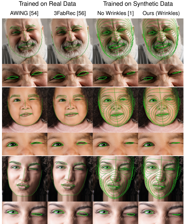
Figure 9: Qualitative results for landmark localization on Pexels. Training on synthetic faces with our expression-based wrinkles is crucial for localizing keypoints in compressed regions of the face.
